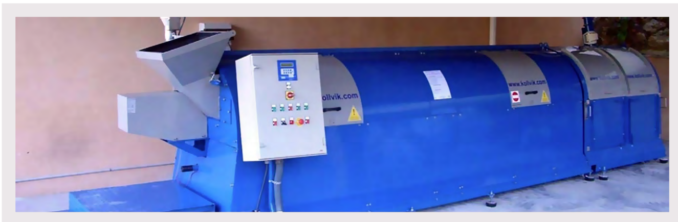
Obrázok 24: Kompostovanie v boxoch technológiou spoločnosti KCS Engineering (zdroj: http://www.kcsengineering.com/rotating-composters-industrial-composting.html )
